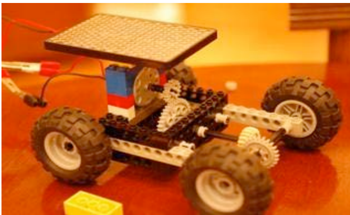
Working solar vehicle with a small gear on the motor and a larger gear connected to a gear assembly on the front axle
