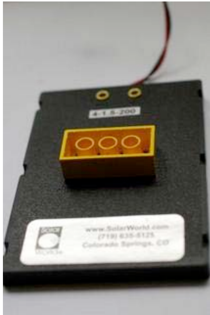
Figure 1. Solar cell with sanded-down Lego pieces glued to back.
