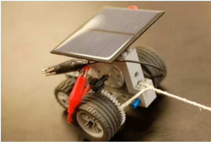
Sample solar vehicle with small gear on motor and large gear connected to axle
